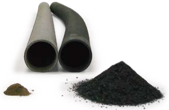
Fig. 4 Comparison of APMT Tube vs. Fe-35Ni-25Cr (after 2300 h at 1100°C). The FeNiCr tube is severely contaminated with oxide flakes.
